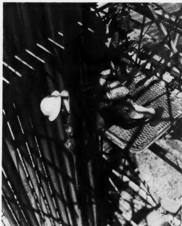
DERRICKMEN have long been accustomed to leaning far off the monkey board to steady the drill pipe as it is screwed up. NOW THE derrickman can rack many thousands of feet of drill pipe with no effort save tilting the control handle in his hand.
